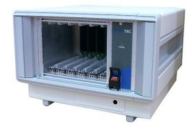
backplane, card guides, pluggable power supply and rear transition area whilst providing the features of IEEE 1101.10 such as EMC, ESD protection, front panel coding and support for inject / extractor handles. The units are shipped assembled, wired and tested with a PICMG 2.11 positronic power interface board, CompactPCI power supply and 5 slot VPX backplane.
