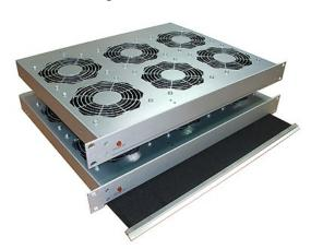
versions are supplied with a front panel mounted power indicator. The standard and filtered fans are available in 3 fan and 6 fan versions and both have 115v ac, 230v ac, 12v dc, 24v dc & 48v dc options. Airflow is up to 120cfm per fan, depending upon the option chosen.
